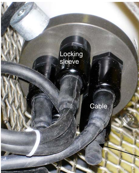
Electronics Control Module shown; verify dummy plug or cable installed for every connector on ECO and CTD
