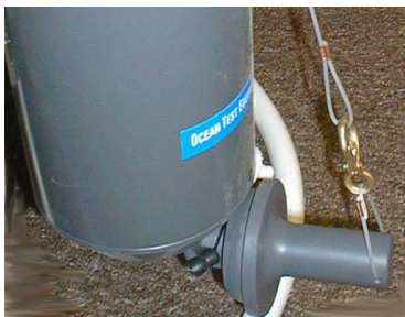
Angling end cap handle away from center of Carousel
