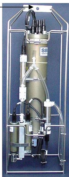
Flat top cage type mounts to CTD extension stand with 50199
