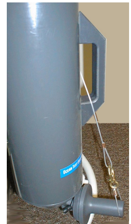
Running middle lanyard through handle
