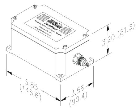
Figure 5. Model 802 *DeepWater* Dimensions in Inches (mm)
