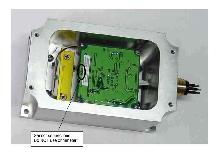
Figure 7. Sensor Connections Inside the Model 802 *DeepWater* Tiltmeter
