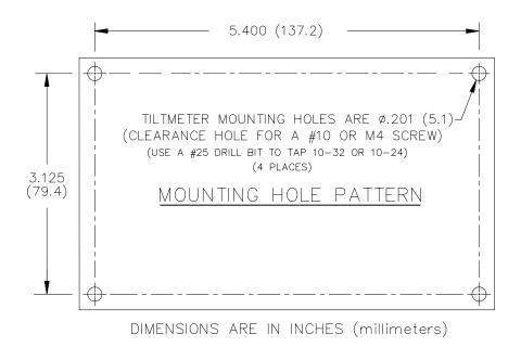
Figure 6. Model 802 *DeepWater* Mounting Hole Pattern
