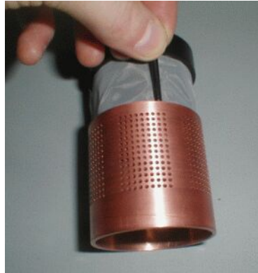
Figure F-5: Start positioning the copper screen
