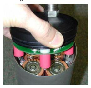
Position the end cap over the open end of the case, with the large springs centered on the battery tops, and the small springs on posts positioned to contact the posts between the batteries. Without rotating the cap, place it on the end of the case.
