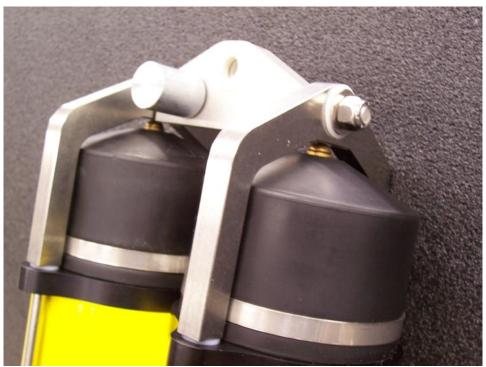
Install part # C980226 Bridge between the two C.A.R.T. units using qty 2 part# 194638 3/8" lock nuts and qty 2 part# 190411 3/8" flat washers.
