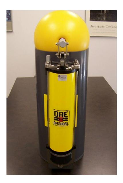
CAUTION: When configured for a pop-up buoy system the CART acoustic release is built with an inverted tilt switch and special "light load" clevis assembly. The release, when configured this way, is rated for a maximum working load of 100Kg.
