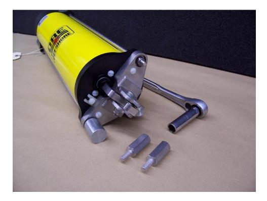
First, start by removing the zinc on the base clevis, next using a 1/2" deep socket remove the two lock nuts on the base clevis. Replace those with qty 2 B980227 standoffs, tighten using an adjustable wrench. Repeat this process on both C.A.R.T.'s
