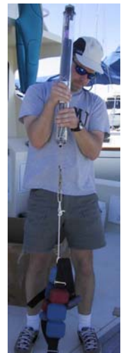
Figure 3.1: 50 lb load test.
