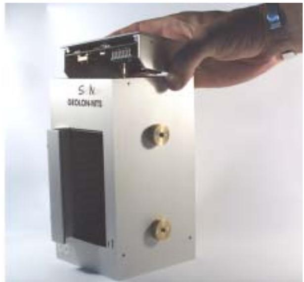
Insert a screw driver into the slot (N0. 10 in chapter 2.2) and twist it to loosen the front plate. Please note that there is a yellow/green grounding wire connecting lid and body, which has to be detached on one end first, before the lid can be taken off completely.
