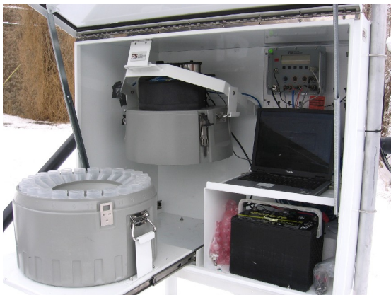
FTS Datalogger with an ISCO autosampler using a DTS-12 for Turbidity Threshold Sampling
