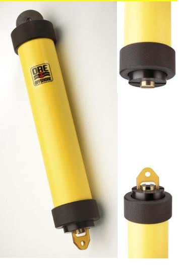
**The SWR** Shallow Water Release is a field-proven, reliable acoustic release. The SWR is made of Delran to avoid dissimilar material issues. The release mechanism is made of Nickel Aluminum Bronze alloy which is excellent for long term deployments. It has been designed for easy use in both in-line moorings and on bottom platforms such as TRBM frames. The SWR is very easy to service and prepare for the next deployment.
