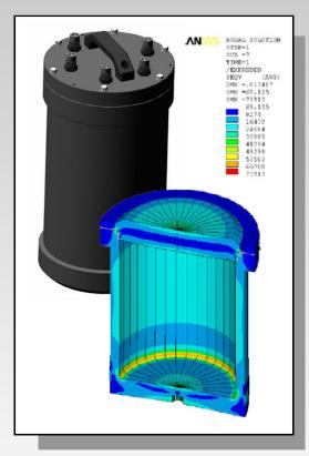
Most enclosures are unique and require detailed stress analysis in order to validate their design integrity. While it is mostly straightforward to correctly size a housing's wall thickness and o come up with early preliminary designs parameters, a sound analysis is crucial in identifying high stress areas due to the interactions of the assembly components.
