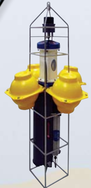
SR-50 with remote transducer head shown connected to an ADCP and CTD, providing real-time data from both instruments.
