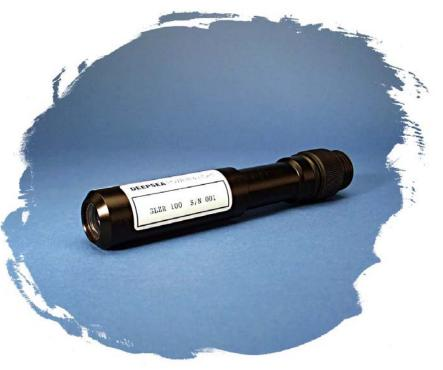
The **SeaLaser**<sup> $^{\text{TM}}$ </sup> 100 is a low cost, lightweight underwater scaling, rangefinding, and aiming device that utilizes a high quality solid state laser diode module. It can be used in pairs or arrays of parallel-aligned beams to determine sizes/scale of viewed objects. Used in an array of three parallel plus one oblique (four total) it can determine zoom lens focal length setting as well.
