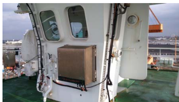
Additional "Top-Box" with independent Air-CO 2 Analyzer LI-7200, GPS and interfaces to meteo. Sensors. Simple data interface to the OceanPack™ system.
