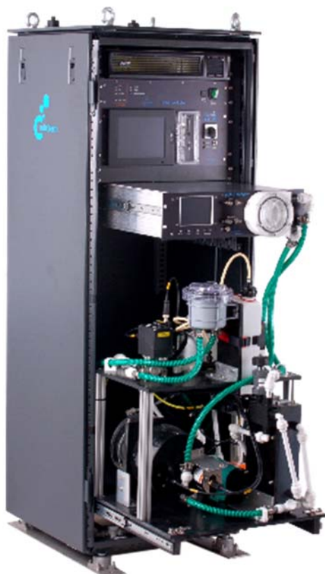
Large pCO 2 "Underway" System with additional sensors, Debubbler and automatic cleaning on a moving drawer
