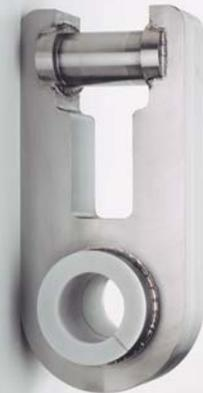
The **HLR Heavy Load Release** is a field-proven, reliable heavy duty acoustic release. The HLR strong back is made entirely of titanium to keep it light and strong. Titanium is also very corrosion resistant. We also use custom made Delran isolation washers to eliminate any risk of dissimilar metals causing corrosion. The HLR has been designed for easy use in both long term moorings and in lowering applications.
