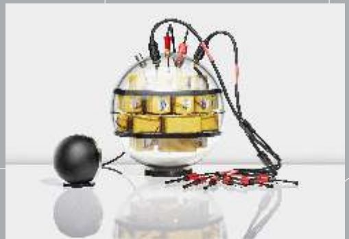
HAM.NODE based telemetry for Modoo with interfaces to 6 different instruments
