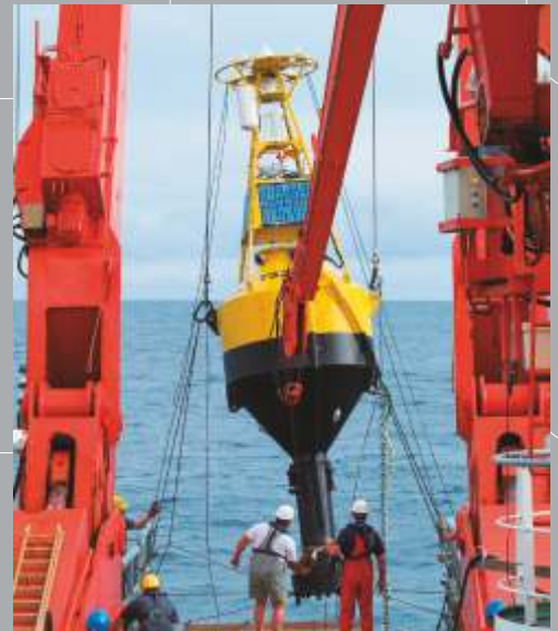
Deployment of GITEWS data buoy with HAM.NODE hydro acoustic data link
