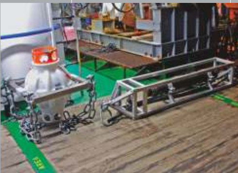
PACT bottom unit (by Optimare) with HAM.NODE OEM modem (left) and HAM.NODE surface modem in custom housing with mooring frame
