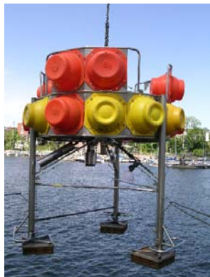
Camera mounted on a tripod for long term deployment. Dr. Peter Linke - GEOMAR
