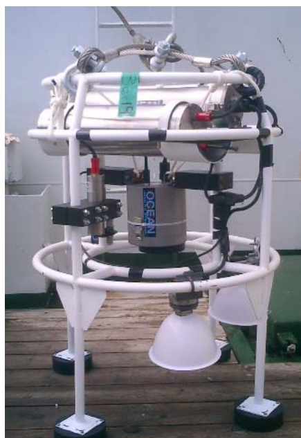
Camera system mounted on a frame for bottom contact (pogo) operation.
