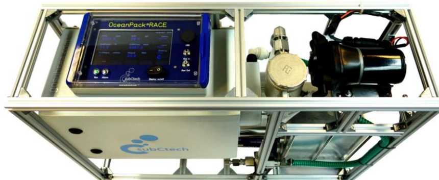
Customized "underway" system for VOLVO OCEAN RACE, with Touch-Display, sea-water supply and sensors
