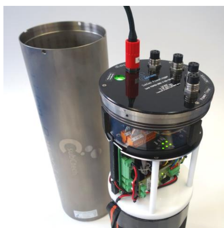
Underwater Data-logger with Li-Ion battery (self-powered, self-recording) and external water-proof Display-Box with 7" Touch-Display for setup and diagnostic. USB port for data download or firmware upgrades
