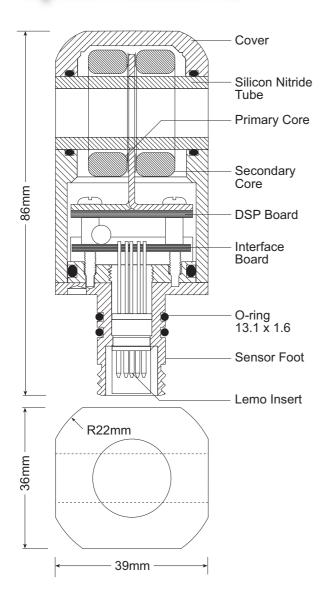
The sensor can be mounted directly on the top end plate of the Aanderaa RDCP 600 and connected to the Sensor Board with a short cable, Sensor Cable 4054.
