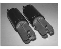
Small portable pair of remote release untis with separate battery pack transponders and Transponder Control Unit (TCU) with Remote Active Transducer (RAT)
