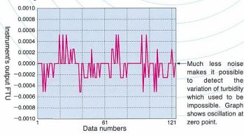
Ultra highly sensitive turbidity sensors have been launched. These sensors have a resolution of 0.0002FTU and their zero point noise is within ±0.0005, which allows accurate measurement in open sea and in deep sea where it used to be hardly possible to measure.
