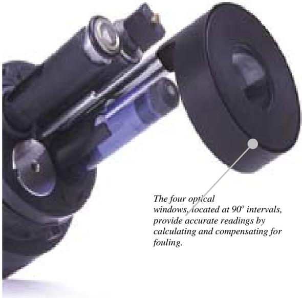
*The four optical windows, located at 90° intervals, provide accurate readings by calculating and compensating for fouling.*
